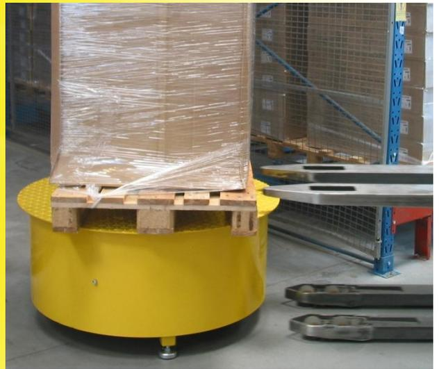
*This pallet turner is completely without any kind of connections, so it can easily be moved to exactly where you need to turn pallets, without use of energy*
