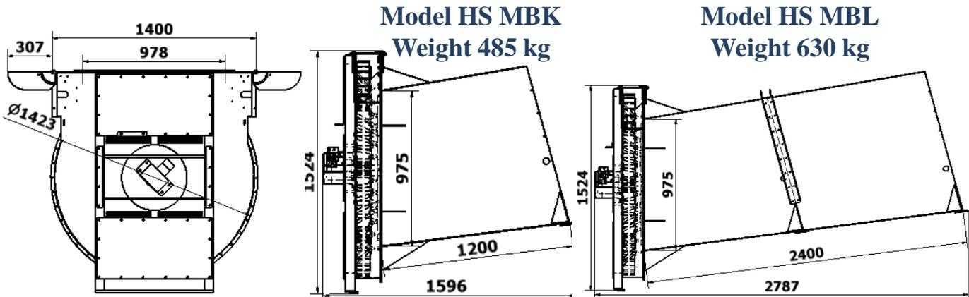
*The Straw Machine is delivered with mounting plate/bracket at customers request, and can be used on all models of loaders, tractors, telehandlers etc.*
